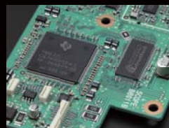
Scope DSP TMS320C6745 by Texas Instruments 32-bit floating point 2250 MFLOPS 370 MHz clock speed
