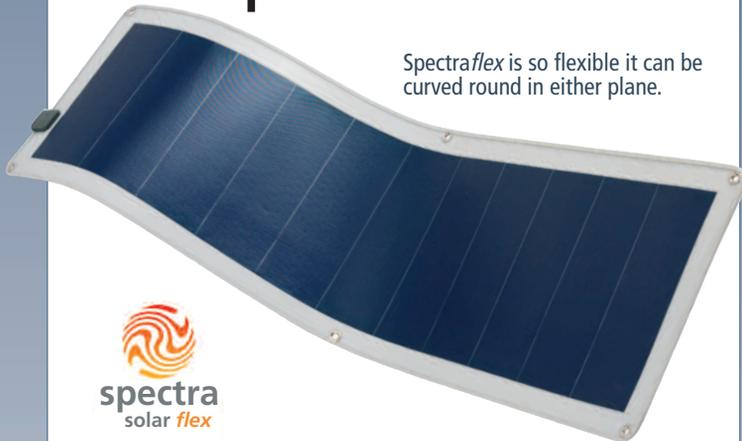
The Spectraflex is a solar panel made from a spectrum splitting amorphous silicon cell design that converts very low levels of light to useable solar energy. Unlike other types of amorphous silicon technology the Spectraflex is very stable over many years where others degrade rapidly soon after deployment. Bypass diodes are connected across each cell so the panel is also shadow tolerant.
